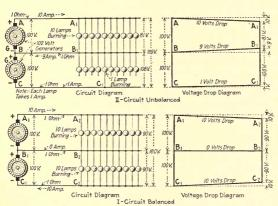
Fig. 99.—Effect of unbalance on a three-wire circuit.
